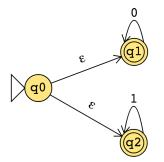
Prune this diagram to get an equivalent DFA with only the "macro-states" reachable from the start state.
